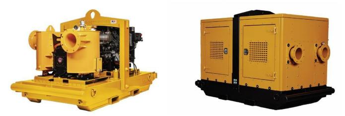
Single Function Pump can ONLY be used for Wellpoint or Sock Drain (clean groundwater, no solids) Applications. Maximum Wellpoint Capabilities: RL-200 (8" Rotary Lobe Pump) is capable of being used on a 700' LF Wellpoint System & (175) 1.5" x 20' FT Wellpoints.
